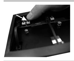
8. The SCS series has the FS-12 pedal, which can be used either as a stand-alone device or as a common bypass device for the whole Pedal Board. In this case it should be placed leftmost on the Pedal Board, while the rightmost place must not be empty. The S3 switch located on the Pedal Board's inner circuit board should be depressed when using the FS-12. In any other case of using SCS pedal in the leftmost position this switch should be pressed down.
